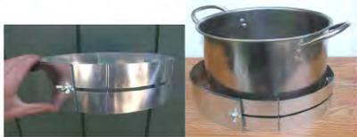
4. Press pot skirt together and tighten screw.
