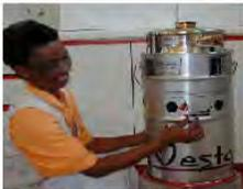
When the food is boiling you can turn down the fire with the control lever to save fuel. The fumes increase when you do this so it is better to use high heat only when indoors. When you have finished
