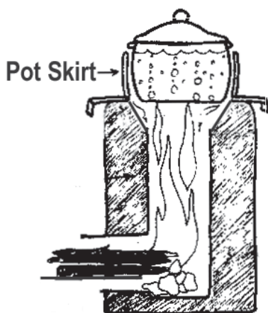
Figure 2 - Appropriate Use of Pot Skirt
